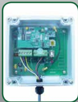
Super Long Range Active (10 to 2000 ft.) for Gate Controls, Personnel/Asset Tracking, Theft Prevention. Wiegand Output, TCP/IP, USB or Serial.
